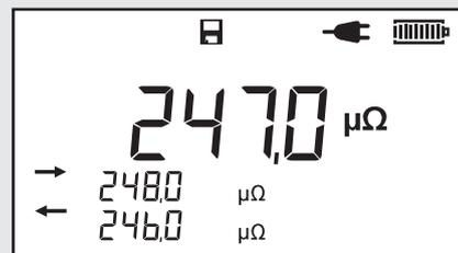
Test results are saved and their memory slot number is shown. The Save screen is shown for three seconds.
