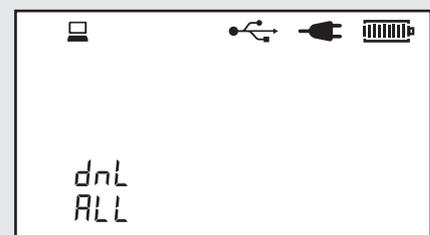
The USB icon
