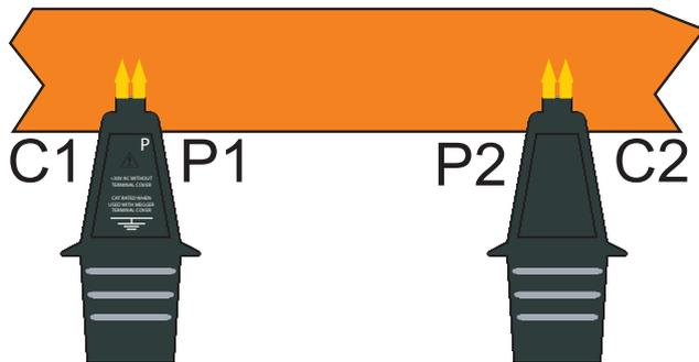
The image shows the correct test lead connection of the current (C1, C2) and potential probes (P1, P2) to a test piece. To make sure test readings are accurate, the current terminals (C1 and C2) must be connected outside of the potential terminals (P1 and P2).
