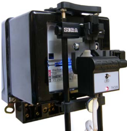
Scanning of rotor marks
