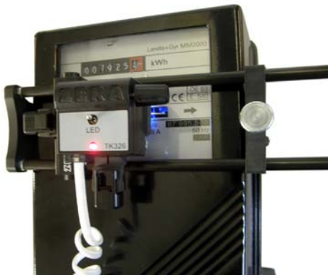
Scanning of rotor marks
