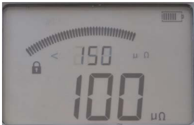
Here P/F limit was set to 150 μΩ and the measured resistance value is 100 μΩ.
